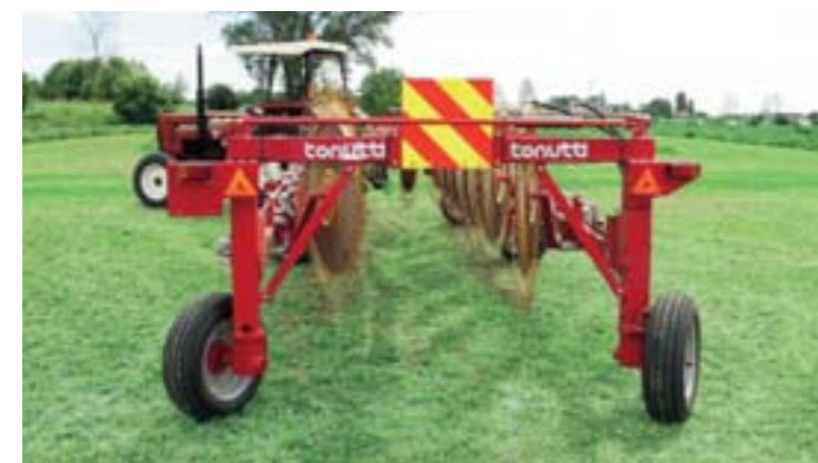
New self-steering mechanism lets the rake perfectly follow the tractor enhancing maneuverability and allowing for tight steering.
