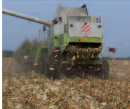
Corn harvesting with built-in stalk chopper.
